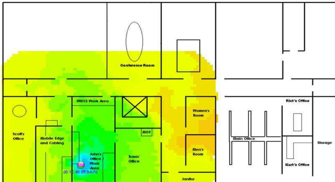
Fig. 3 1059-00 Site Survey Test with Cisco 1242 at 2 dBm Tx Power (August 17, 2010) 5 GHz without enclosure
