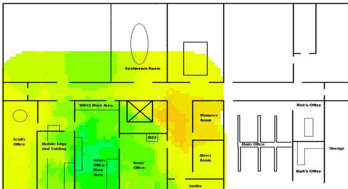
Fig. 4 1059-00 Site Survey Test with Cisco 1242 at 2 dBm Tx Power (August 17, 2010) 5 GHz with enclosure
