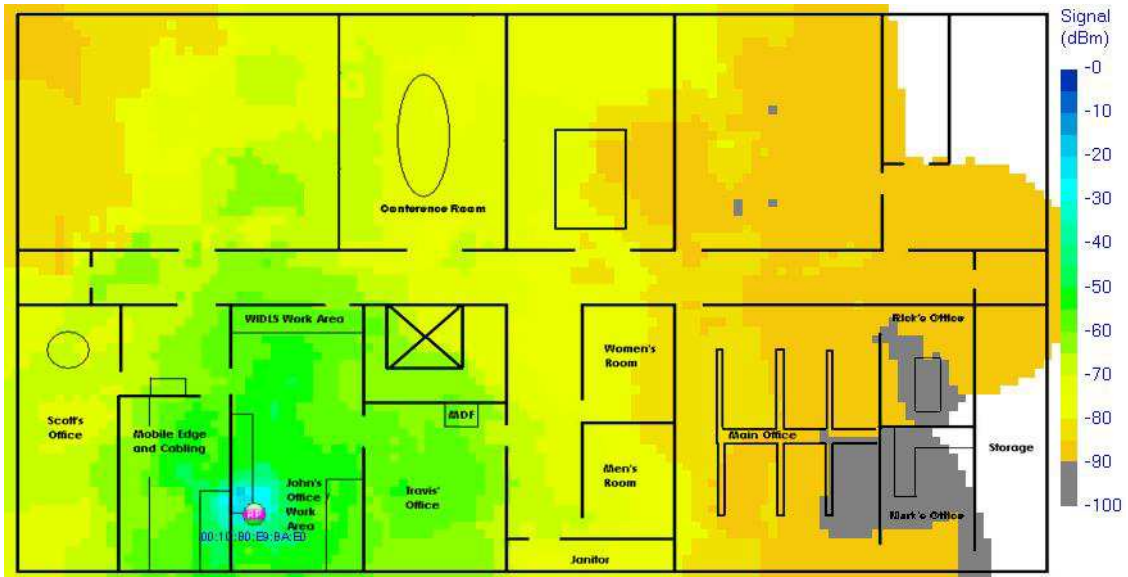
Fig. 1 1059-00 Site Survey Test with Cisco 1242 at 2 dBm Tx Power (August 18, 2010) 2.4 GHz without enclosure
